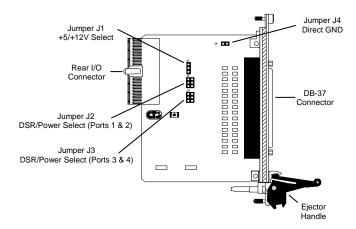
Figure 4: Titan/cPCI Rear I/O two and four port adapters
